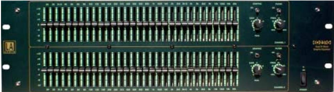
31 band pass filters based around precision minimum phase active RC networks deliver superior dynamic range and signal to noise performance. 45mm long throw faders provide maximum sensitivity and control of 12dB cut and boost at ISO centre frequencies from 20Hz to 20KHz.
